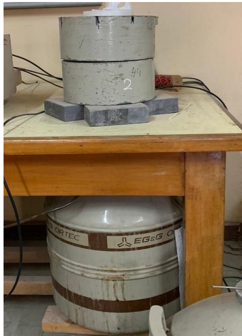
Figure 2: Experimental measurements of \gamma -ray attenuation coefficient
