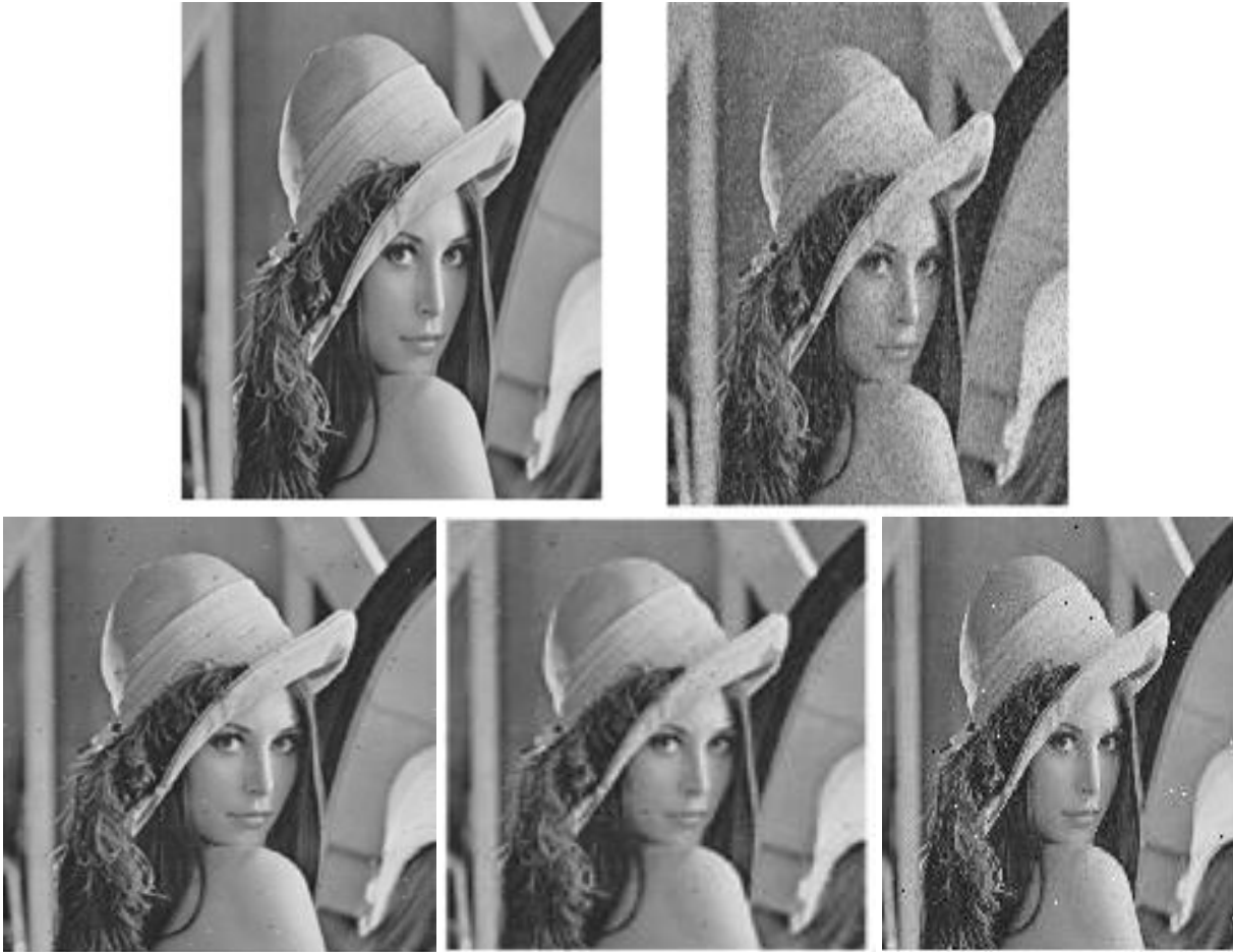
Figure (a).original gray scale lena image.Figure (b).lena image corrupted by 40% impulse noise. Figure (c).this image represent the filter outputs of the 3x3 matrix scanning fuzzy logic based. Figure (d). after apply the 3x2 and 4x4 matrix scanning fuzzy logic based. Figure (e) represent the better quality image and remaining noise is filtered by using the soft thresholding concept.
