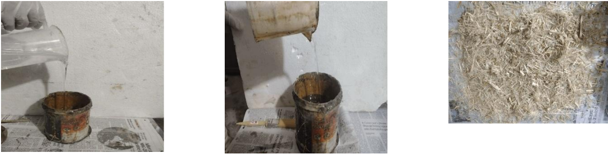
Fig. 3. Fabrication sequence: (a) and (b) epoxy resin mixing and preparation; (c) resin application onto fibre layers during hand lay-up consolidation.
