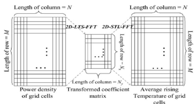
Fig .3. Overview of using 2D-SLT-FFT and 2D-LTS\_FFT to evaluate the average rising temperature of grid cells.
