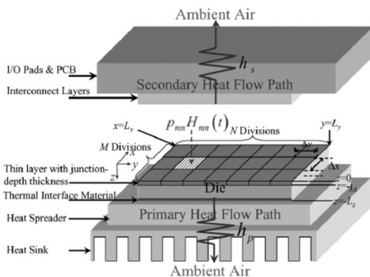
Fig. 1. Compact thermal model for early design stages
