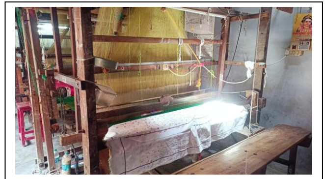
Fig.3. Handloom setup to weave a pure Kanchipuram silk saree
