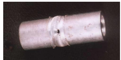
Fig. 4 A photograph of the keyhole remained after ending the FSW process.
