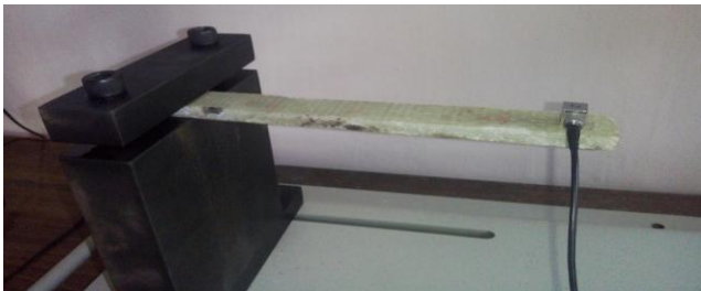
Fig 6. Cantilever Beam Test set up
