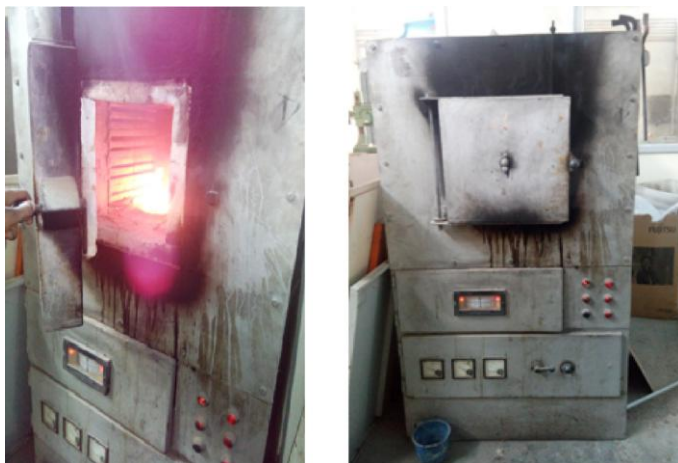
Fig 3. Burn out test using furnace
