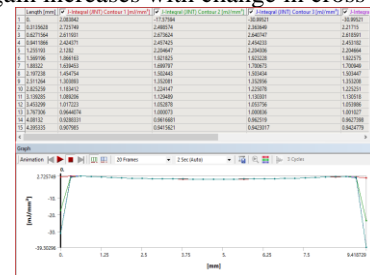
Fig 5.22: The graph shows between J-integral (energy distribution) and length (mm) at (R=2)
