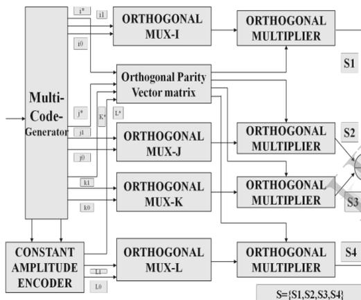
Figure.4. Biorthogonal Encoder
