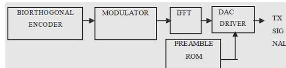
Fig 3: Overall architecture of MIMO-OFDM baseband Transmitter to use 8-way parallel data-paths.
