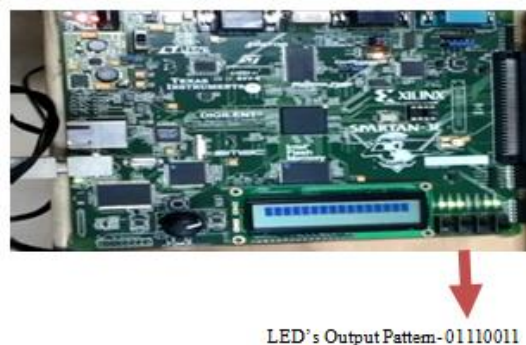
Fig.16. Output of Morphology Dilation operation on Spartan 3E-XC3E-500-4FG320 Evaluation board
