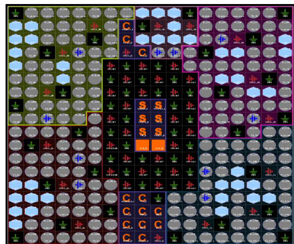
Fig. 7 Synthesized FPGA device view showing the target SPARTAN-7 (xc7s50csga324-1) package and available FPGA resources used for implementation of the DAQ system
