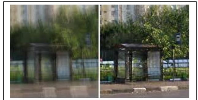
Fig 3. Example for Weiner deconvolution method a) Blurred image b) Deblurred image
