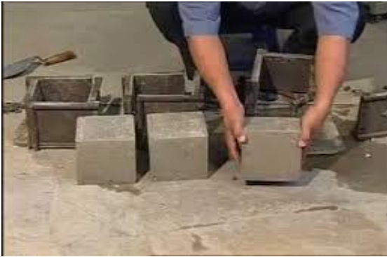
Fig-5. Sample of Concrete Cube
