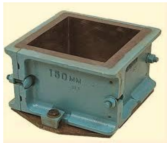
Fig-4. Mould of concrete cube
