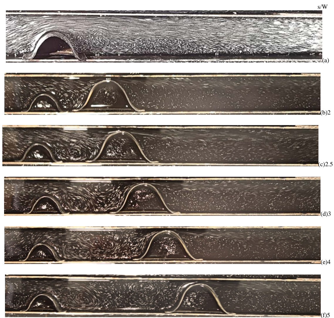
Fig.9 Flow pattern for r/W=0.5 , r_i/W=0.9 , for various s/W ratio.
