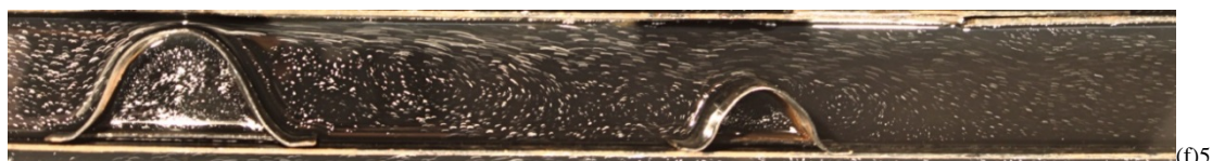
Fig.13 Flow pattern for r/W=0.9 , r_f/W=0.5 , for various s/W ratio.
