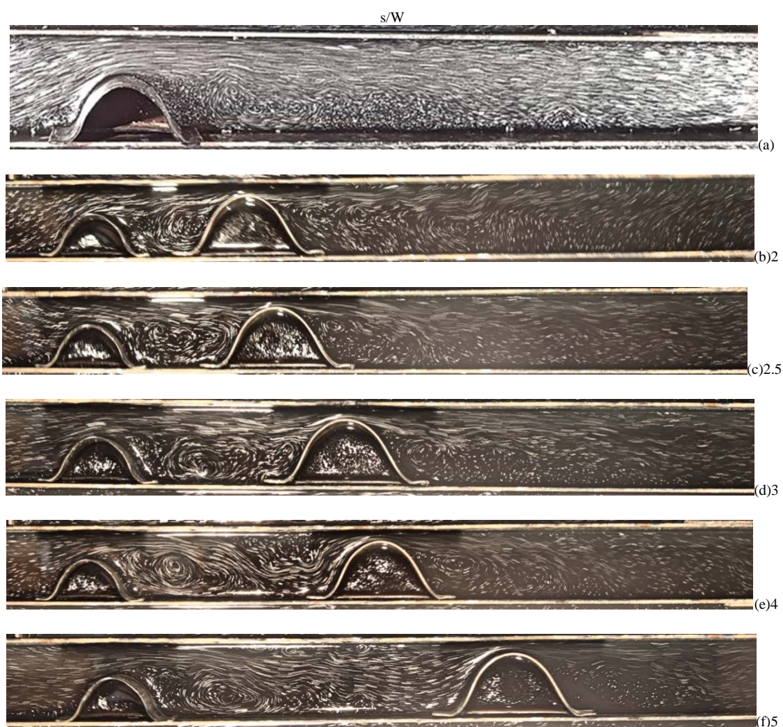
Fig.8 Flow pattern for r/W=0.5 , r_i/W=0.75 , for various s/W ratio.
