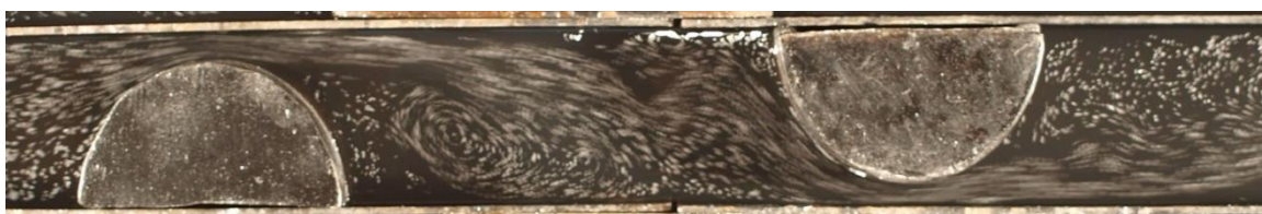
Fig 15: Flow pattern for r/W=0.9 , r_t/W=0.9 , for various s/W ratio.
