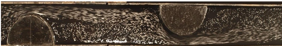
Fig.11 Flow pattern for r/W=0.75 , r_1/W=0.75 , for various s/W ratio.
