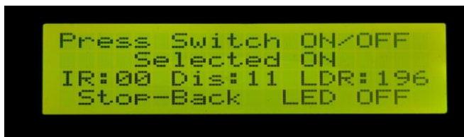
Fig 15: Backward motion (Ultrasonic) in Autonomous Mode
