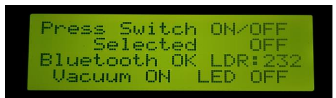
Fig 20: Vacuum motor ON in Manual Mode
