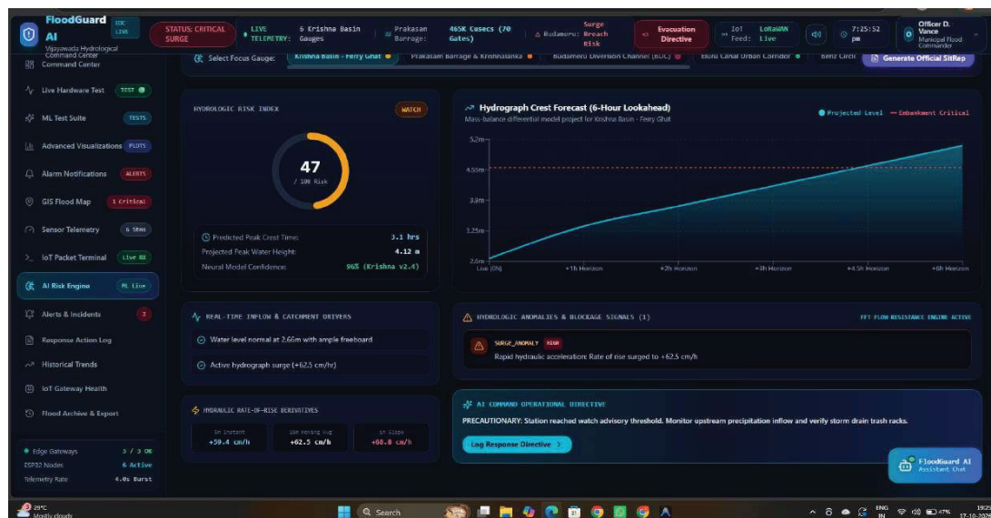
Fig. 11. AI risk-engine view for ST-001: gauge, six-hour hydrograph projection, drivers, surge anomaly and directive (injected scenario).
