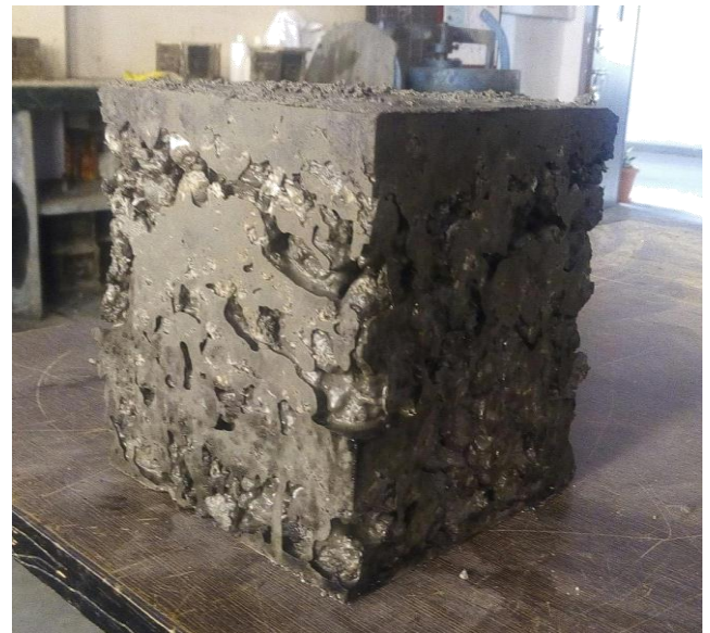
Fig.1: Cube showing rough surface
