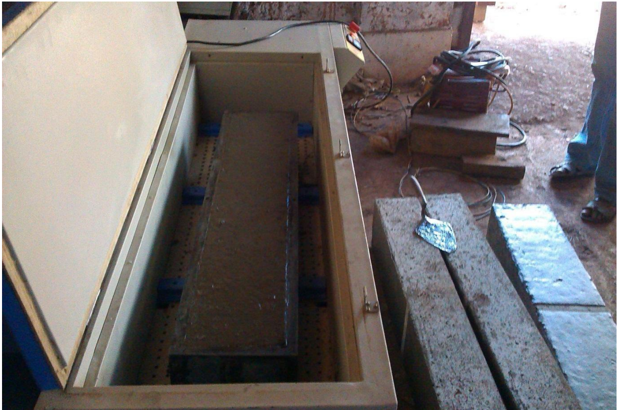
Fig. 3.9: Casted specimen placed in hot air oven for curing.
