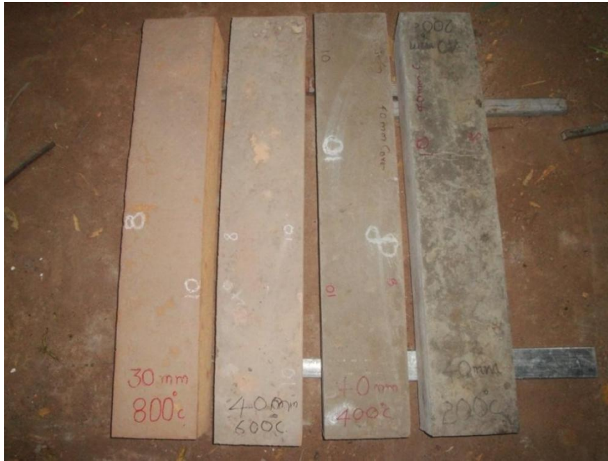
Fig. 3.14: Colour variation in the specimens after heat treatment
