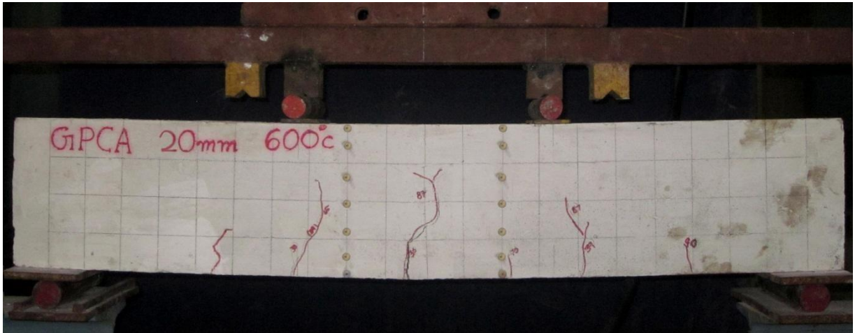
Fig. 4.20: Crack pattern of GPCA 20mm 600°C
