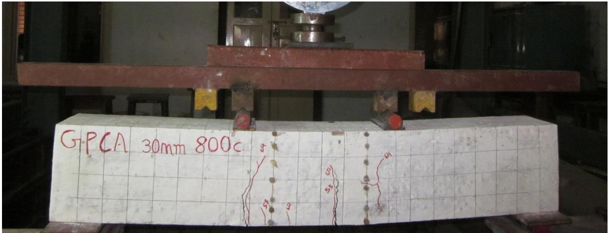
Fig. 4.26: Crack pattern of GPCA 30mm 800°C
