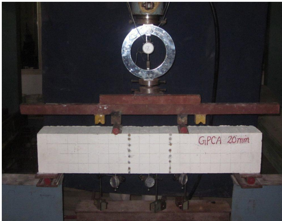
Fig. 3.19: Flexural Strength testing of geopolymer beam specimen.
