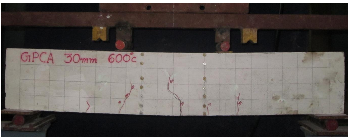
Fig. 4.25: Crack pattern of GPCA 30mm 600°C
