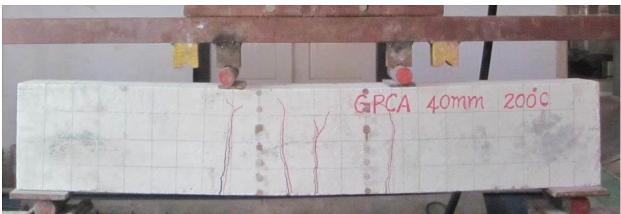
Fig 4.28: Crack pattern of GPCA 40mm 200°C
