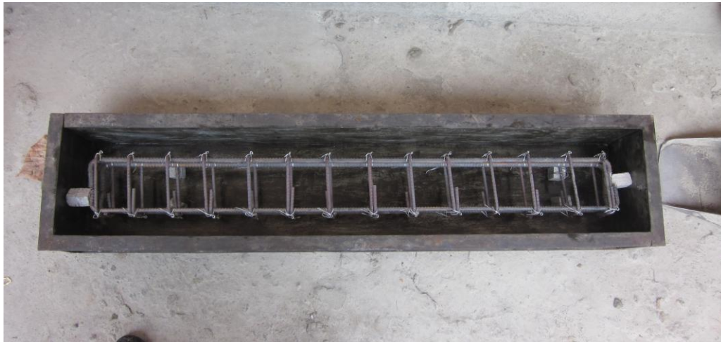
Fig. 3.7: Casting of 40mm beam specimen
