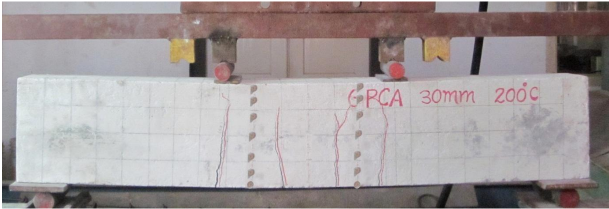
Fig. 4.23: Crack pattern of GPCA 30mm 200°C
