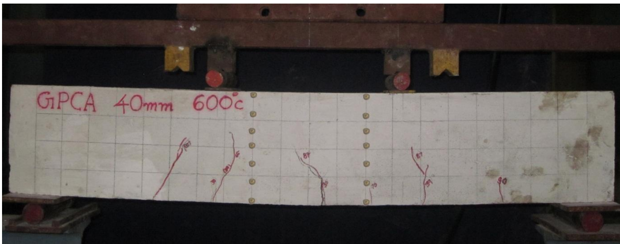
Fig 4.30: Crack pattern of GPCA 40mm 600°C
