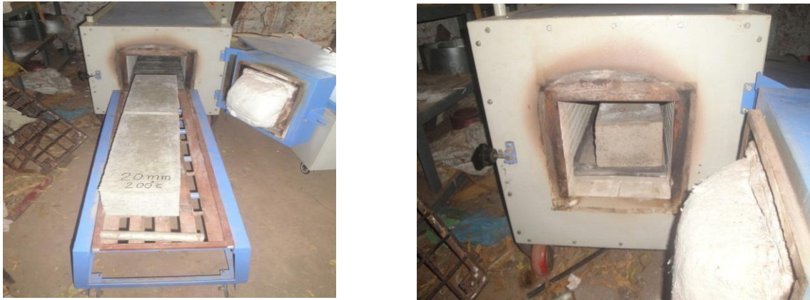
Fig. 3.11: Cured beam placed in the furnace
