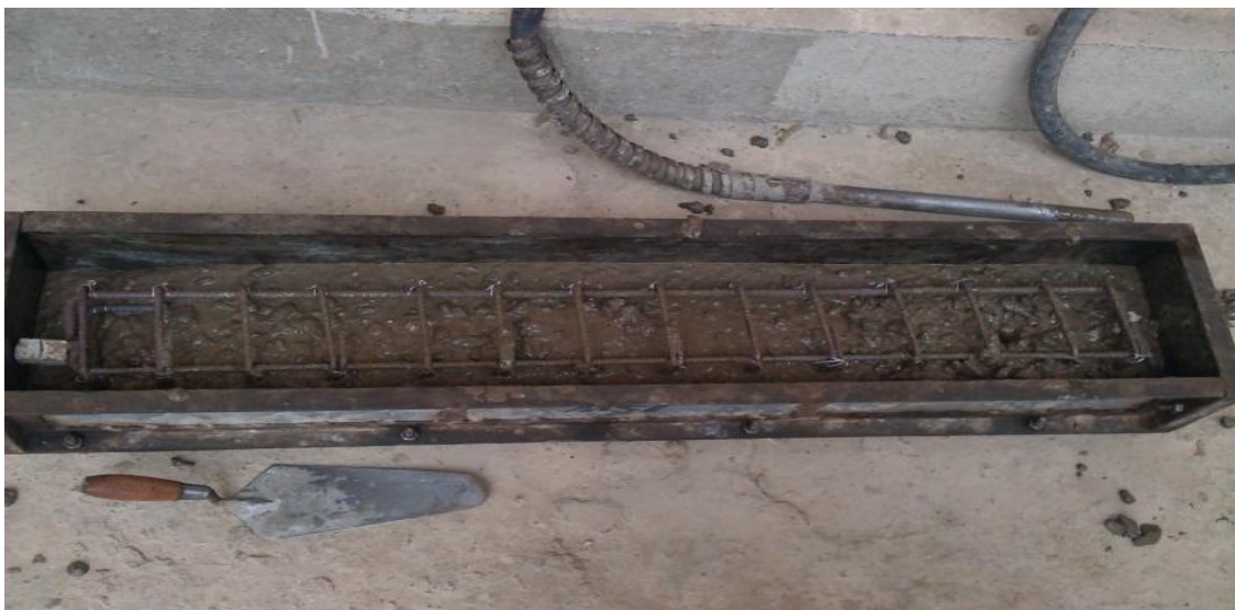
Fig. 3.6: Casting of GPC 30mm beam specimen
