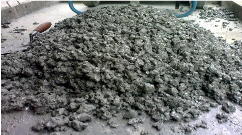
Fig. 3.4: Geopolymer concrete after mixing
