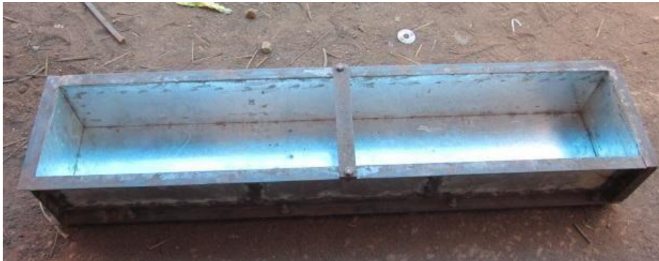
Fig 3.2: Mould for Beam casting
