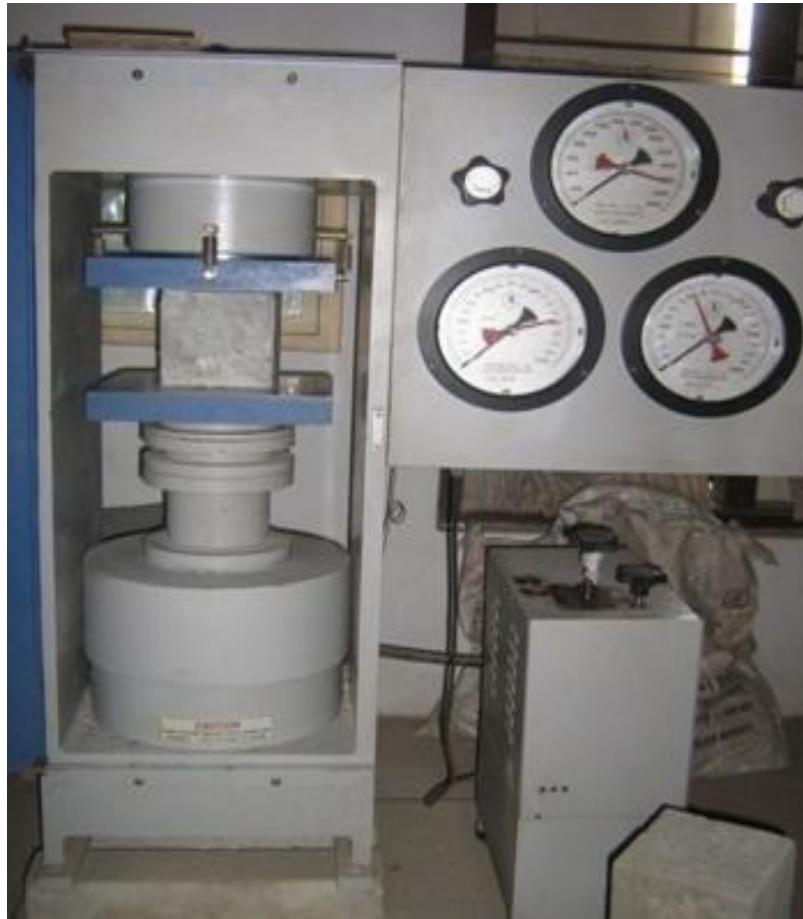
Fig. 3.17: Compressive strength test on GPC cube
