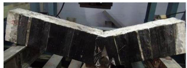
Fig. 9. Rupture of the CFRP sheet in the series #5 beam
