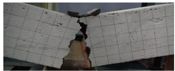
Fig. 6. Flexural-brittle failure of series #1 beam
