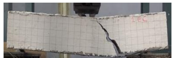
Fig. 8. Shear failure of the series #3 beam
