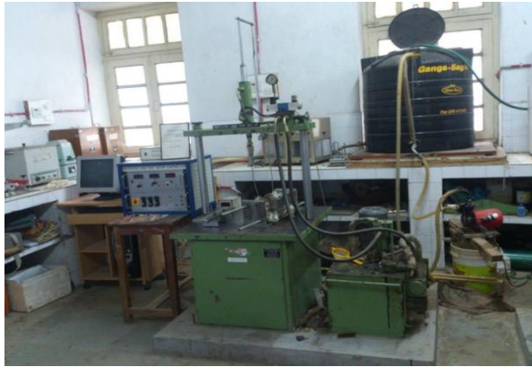
Fig. 1: Flexural fatigue test setup
