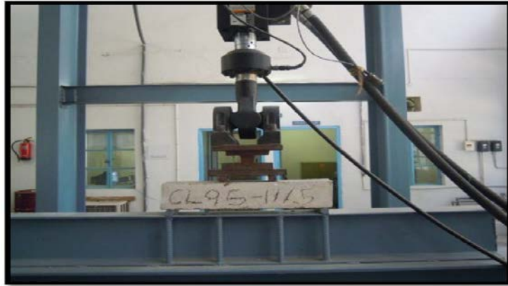
Plate: shows the set up for static flexural and flexural fatigue tests.
