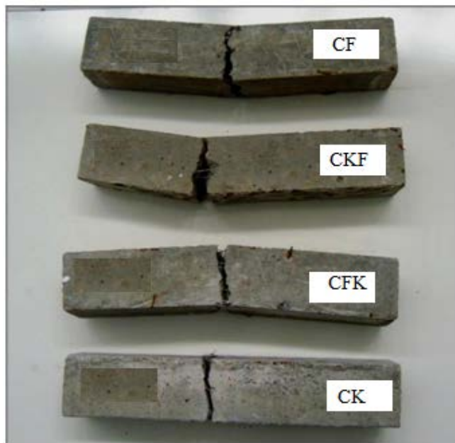
Plate:- The typical failure pattern in control and SF based concrete specimens under fatigue loading.
