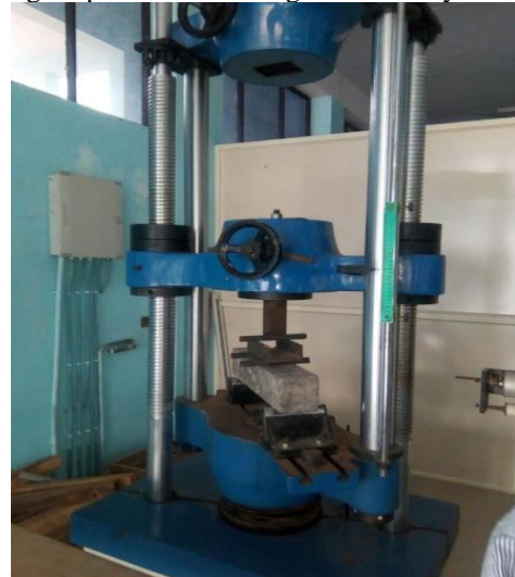
Fig.3 Flexural Strength Test on Beam
