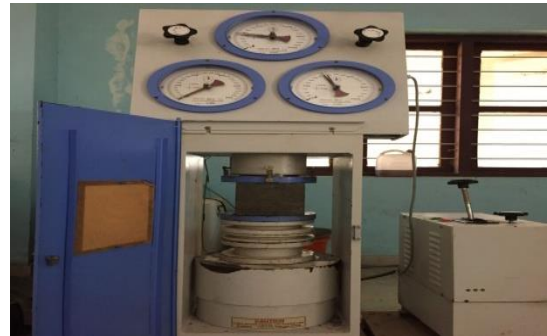
Fig.1 Compressive Strength Test on Cube
