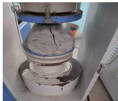
Fig.2 Split Tensile Strength Test on Cylinder
