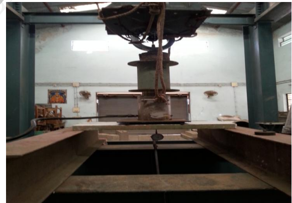
Fig 2: Test setup of specimens under flexural loading
