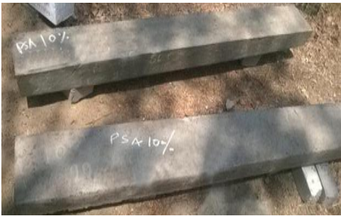
Fig. 5 Sun light Curing of GPC Specimens
