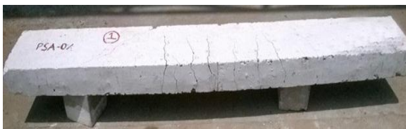
Fig. 20 Crack Pattern of GPC 0 % Sun Light Cured Specimen.
