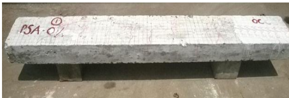
Fig. 18 Crack Pattern of GPC 0 % Oven Cured Specimen.
