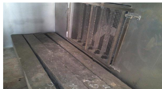
Fig. 4 Oven Curing of GPC Specimens.
