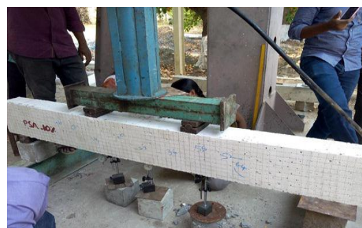
Fig. 8 Two Point Loading Setup
