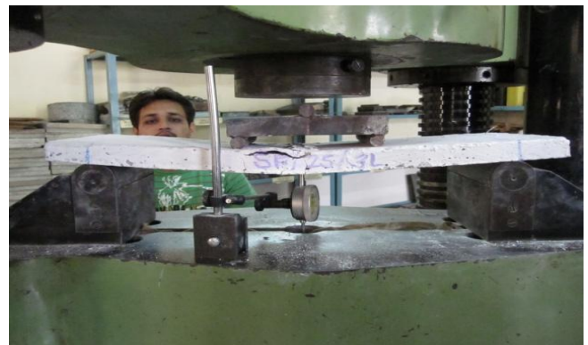
Fig 11. Showing (25mm- 3 layer) panel failure
