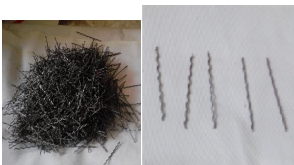
Fig 3-Corrugated type steel fibers with aspect ratio (l/d) =57
