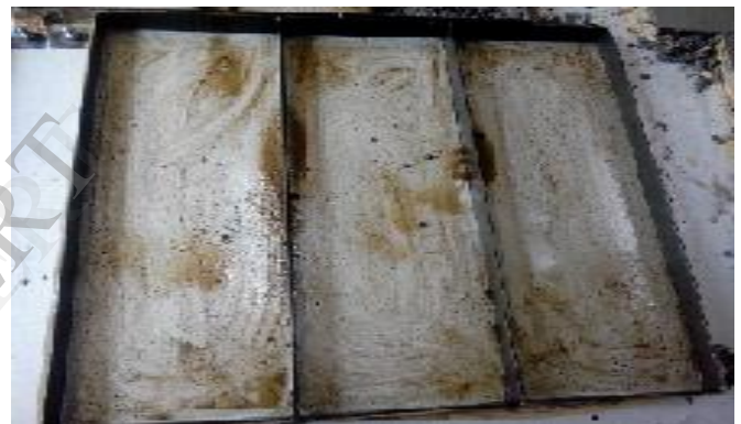
Fig 5-Steel mould oiled before casting of thickness 25 mm
