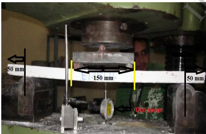
Fig 8-(25 mm-2 layers) panel under testing set-up
