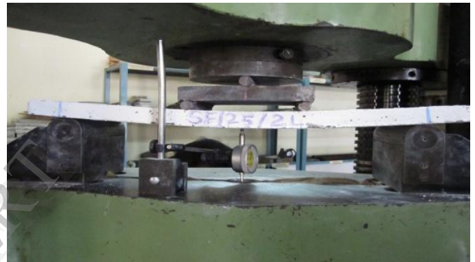
Fig 10. Showing (25 mm-2 layer) panel failure
