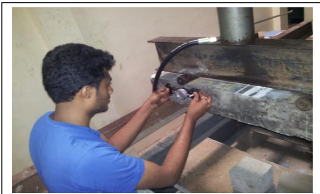
Fig 3. Strain measurement using demec gauge
