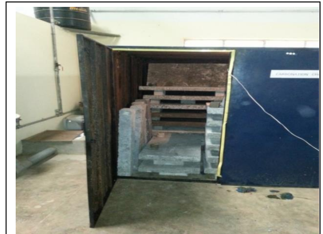
Fig 1. Beams inside carbonation chamber
