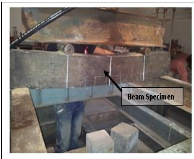
Fig 4. Strain measurement using demec gauge
