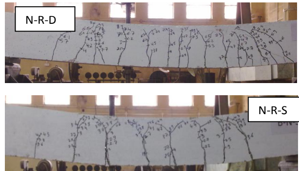
Figure 15: Crack pattern of reference beams
