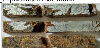
Fig. 2: Failed specimen in bending test
