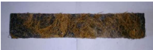
Fig. 1: ASTM-recommended flexural test specimen
