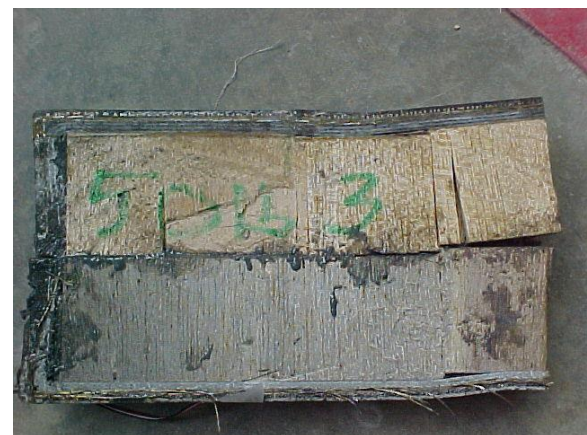
Fig. 26. Core shear failure and transverse shear failure
