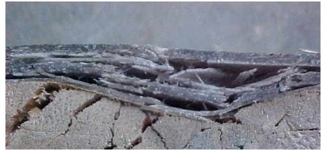
Fig. 16. Interfacial debonding and core shear failure
