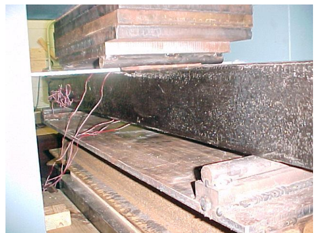
Fig. 3. Side view of specimen, strain gauge wire and LVDT attachment for a 3-point bending test
