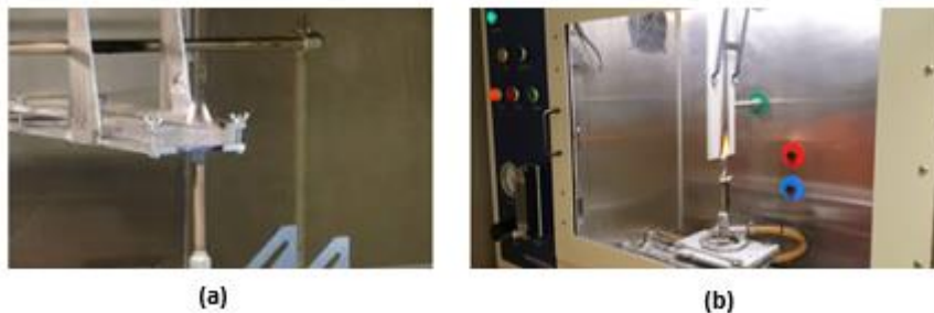
Fig.1 Illustration of horizontal and vertical flame testing setup
