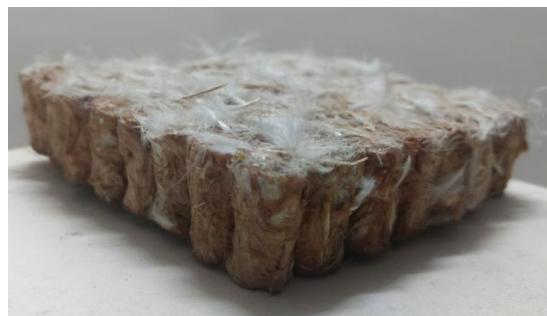
Figure 4: FECORE - Feather fiber based hybrid honeycomb core [8]
