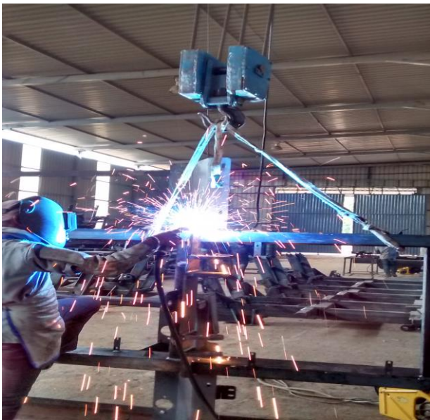
Fig.3 The Chassis is rotated 90 Deg & Held in over head crane to full vertical weld position.
