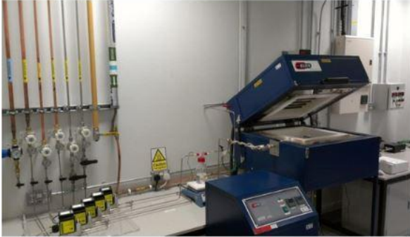
Fig 2.1 Electric heater furnace, Control furnace panel, Bubbler and Mass flow controllers
