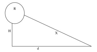
$$\begin{split} X &= \sqrt{H^2 + d^2} - R \\ &= \sqrt{(20.51)^2 + (10)^2} - 13.67 \\ &= 9.147 \text{ m} \\ F, \text{ View factor} &= D^2/4(r+x)^2 \\ &= (27.35)^2/4(13.67 + 9.147)^2 \\ &= 748.022/2082.461 \\ &= 0.35(\text{View factor}) \\ Ep, \text{ Emissive power} &= \Pi \times M \times H_c/\pi \times D^2 \times t \\ &= 0.25 \times 110 \times 46000/\pi (27.35)^2 \times 2.84 \end{split}$$
