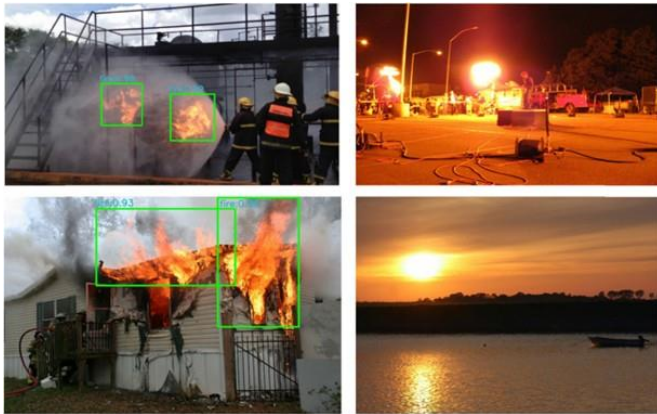
Fig. 5: Detection results guided by GIN: (a) flame in a factory (top left); (b) street with artificial light sources (top right); (c) burning house (down left); (d) river in sunset (down right).
