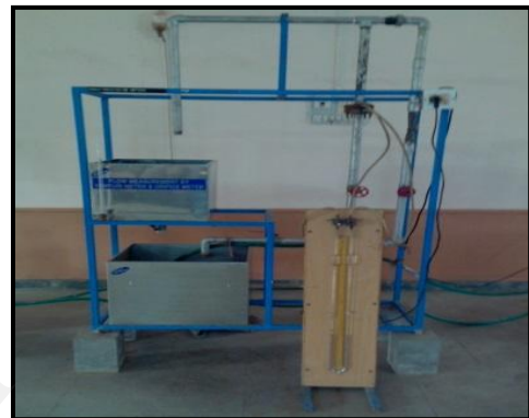
Fig 2: Experiment set up of Orifice meter
