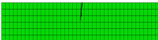
Fig.6: Example of Cracking propagation at FE beam
