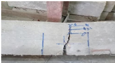
Fig.5: Example of Cracking propagation of experimental beam
