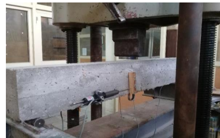
Fig.2: Test Specimen beam under loading
