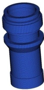
Fig.1 Solid model of diesel generator cylinder
