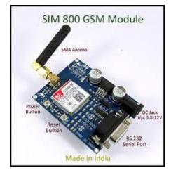
This module will settle for any GSM network operator SIM card. Advantage of this module is that we are able to use RS232 port to speak. This GSM electronic equipment is extremely versatile plug and play quad band GSM electronic equipment for direct and simple integration to RS232 applications. GSM module uses customary AT Commands
