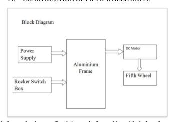
All four wheels are fixed in each four side with help of dummy wheel. In dc motor rocker switch wiring are solder and rocker switch give connection on external sources. The fifth wheel are attached to aluminium frame with dc motor.
