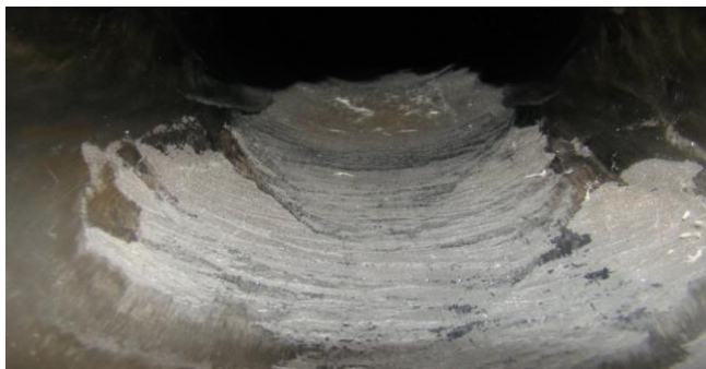
Fig 1. Defective barrel showing sintered sand particles
