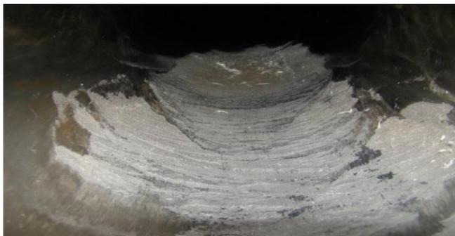
Fig 1. Defective barrel showing sintered sand particles
