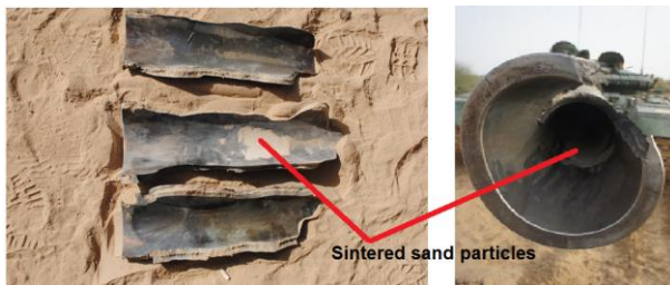
Fig 2. Failed gun barrel showing presence of sintered sand particles
