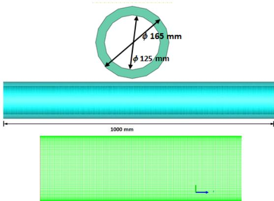
Fig. 3 Barrel dimension and meshing
