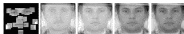
Figure 3. Illustration of iterative PCA reconstruction. After initializing with the patch face reconstruction (leftmost image), we iteratively refine the estimate using successive projections onto the face subspace. Iterations shown are t = 0, 5, 100, 500 , and 1000
