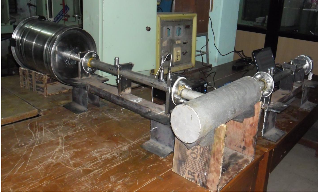
b. Configuration with load Fig. 4 Experimental setup for two load method
