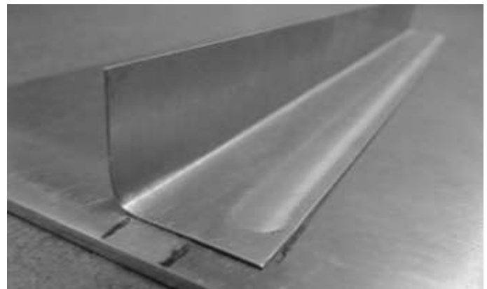
Figure 7. A thin angle plate friction stir welded to thicker plate without the need of mechanical fixation
