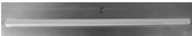
Figure 6. A typical thin sample joined by FSW with conjunction with adhesive fixing technique
