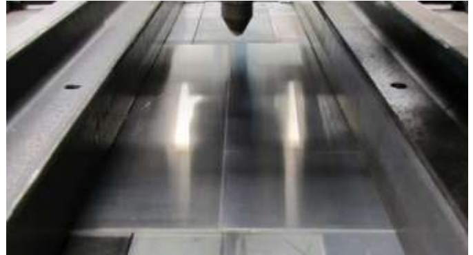
Figure 3. Simplified mechanical clamping with steel U-profiles for alternative adhesive fixation
