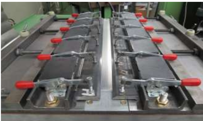
Figure 2. Conventional mechanical clamping with a hold-down construction
