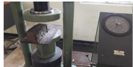
Fig. 3 : Compressive Strength on plastic brick
