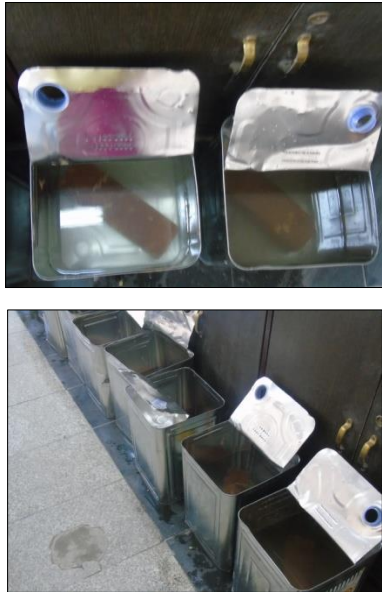
Fig 2: Water Absorption of bricks
