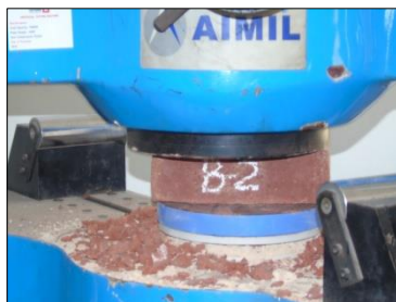
Fig 3: Compression Test on UTM
