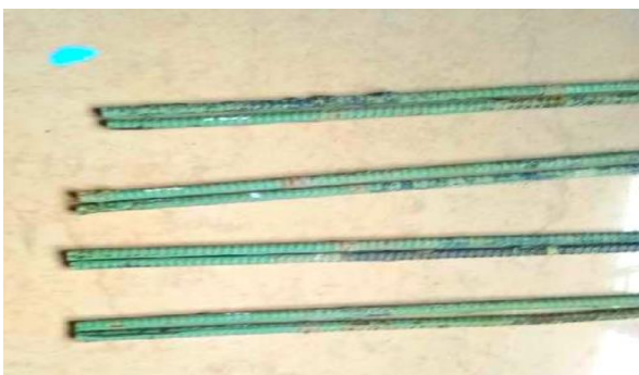
Fig.5. Reinforced bars after ACT
