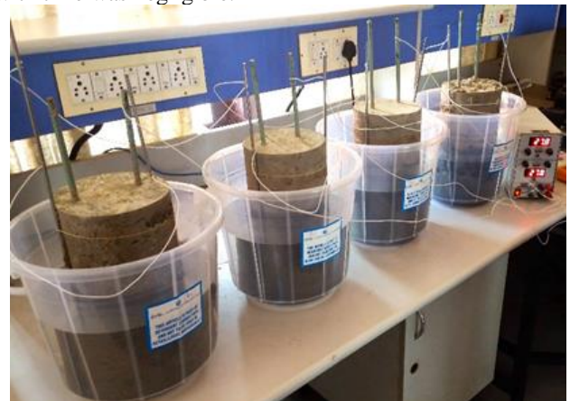
Fig.4. Laboratory setup of accelerated corrosion test
