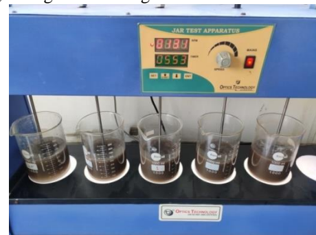
Fig.no.06: Flocculation by using jar test apparatus.
