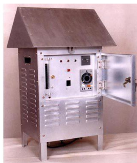
Figure Error! No text of specified style in document..2 Pictorial View of High Volume Air Sample
