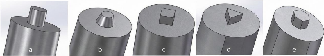
Figure 3 FSW tools with different pin profile (a) cylindrical; (b) tapered cylindrical; (c) triangular; (d) square and (e) hexagonal.
